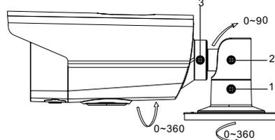
Figure 2-7 3-axis Adjustment
