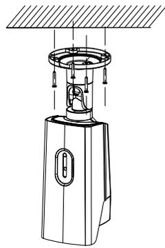
Figure 2-6 Fix the Camera to the Ceiling
